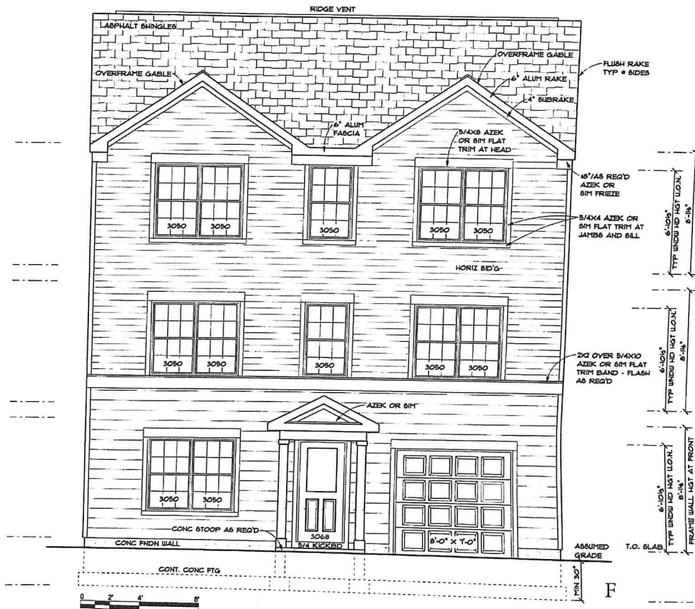
Front Elevation at Slab-on-Grade Condition SCALE: 1/4" = 1'-0"
