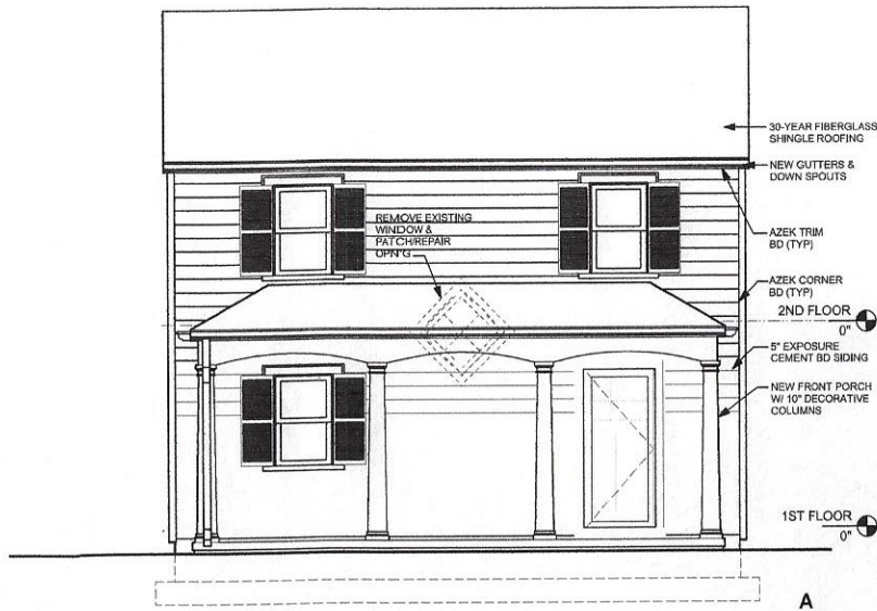
1 PROPOSED FRONT ELEV Scale: 1/4" = 1'-0"
